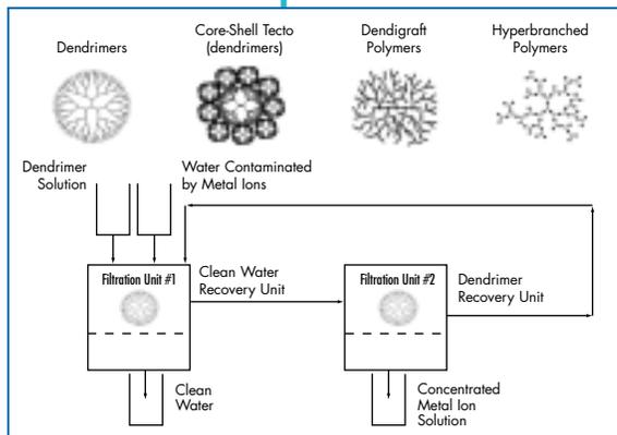
Recovery of metal ions from aqueous solutions by dendrimer-enhanced ultrafiltration. Reprinted with permission from *Environmental Science and Technology*, 2005, 39, 1366-1377. Copyright 2005 American Chemical Society.
