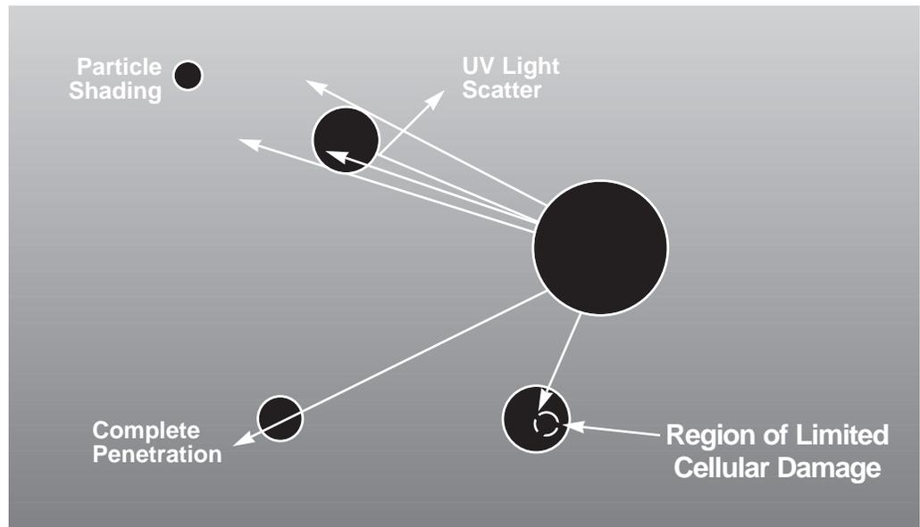
**Figure 1.** Impact of particles on UV light transmittance.
