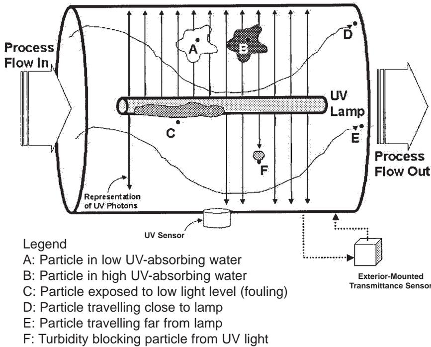
**Figure 2.** Water quality and process variables creating differences between applied and transferred UV dose.
