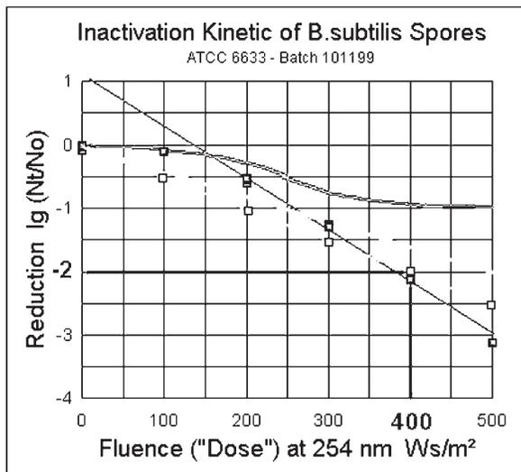
**Figure 3.** “Shoulder-Curve Kinetic” is more sensitive to detect hydraulic and irradiance deficiencies than is “Linear Kinetic” because fractions obtaining “Doses” below 100 J/m<sup>2</sup> are not inactivated and contribute fully to lower lg-reduction results. Example: 10 percent receives less than 100 J/m<sup>2</sup>.
