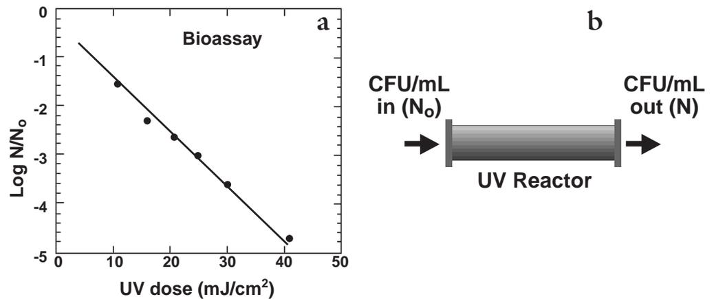
**Figure 1.** Schematic of a biodosimetry test. (a) A relationship between applied UV dose and log survival of the challenge organism is developed under controlled laboratory conditions — measurement of UV dose is traceable back to NIST standards. (b) Challenge organism is seeded into UV reactor. The log of the ratio of surviving organisms to initial organisms is calculated and a reactor UV dose is determined from the plot in (a).
