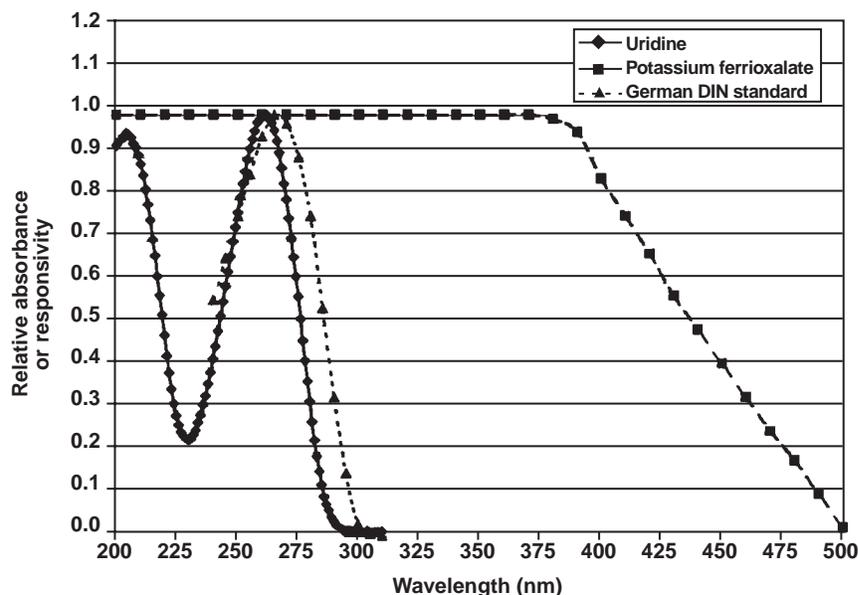
**Figure 3.** Absorbance spectra of uridine and potassium ferrioxalate, and responsivity of the German DIN Germicidal Standard.
