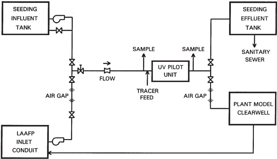
Figure 2. UV pilot study schematic.
