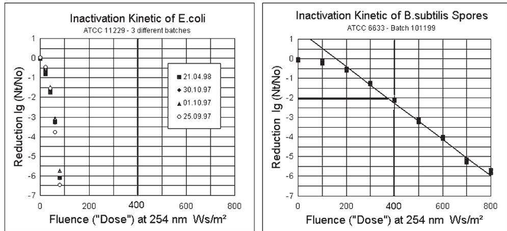
Figure 1. *E.coli* is no suitable organism to test for 400 J/m<sup>2</sup>, but *B. subtilis* spores are.
