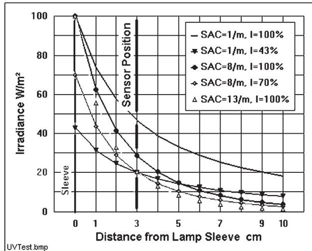
**Figure 4.** Diagram to explain why a UV-System — example: setpoint 20W/m<sup>2</sup> good for SAC = 8/m and 70 percent lamp intensity — must be tested with two settings. In this case, ▼ SAC = 1/m, I = 43 percent. △ SAC = 13/m, I = 100 percent.
