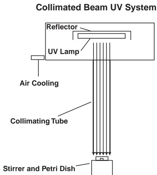
**Figure 2.** Collimated beam UV apparatus used on the bench scale to develop standardized dose-response data for microorganisms.
