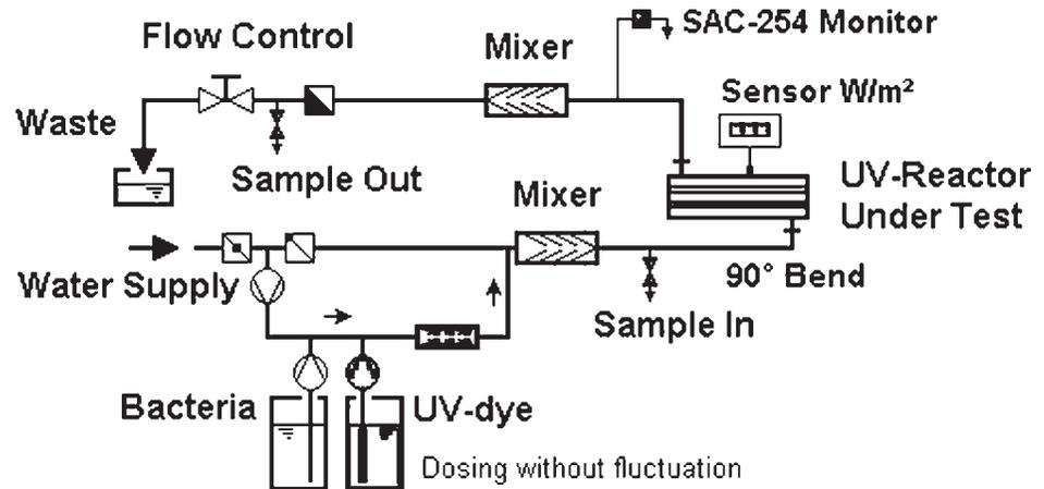
Figure 2. Test facility for UV-Systems acc. to DVGWW 294.
