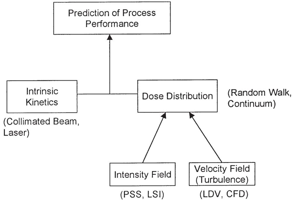
**Figure 1.** Schematic representation of dose distribution model components. Parenthetical entries refer to methods that have been used to measure or model each component. Arrows indicate the direction of information flow and integration in developing estimates of process performance.
