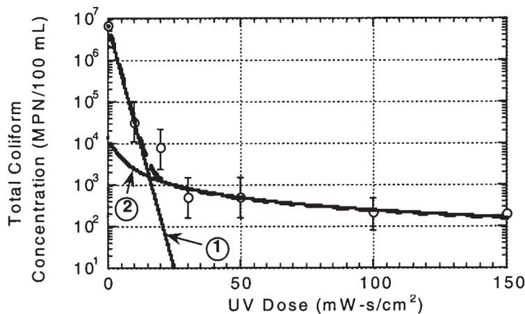
**Figure 2.** Graphical representation of the UV disinfection model developed to describe both the first order kinetic and tailing regions.
